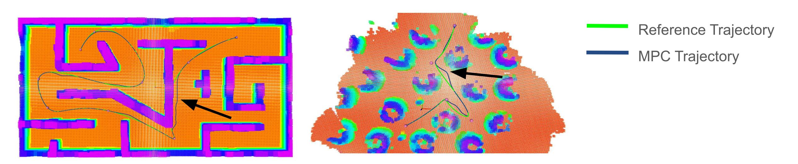
Dynamic Obstacle Avoidance - Avoiding moving objects by considering both dynamic and static obstacles The result shows the screenshot of two time step in one video. When a dynamic obstacle appears in the reference trajectory, by applying both static obstacles and dynamic obstacles constraints, a safe trajectory is generated.
